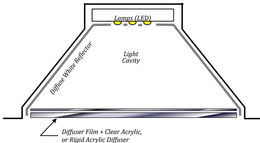
Figure 1. A Typical LED Down Light
